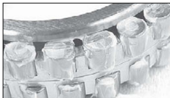
Fig. 2: Grease Packed Cylindrical Roller Bearing
