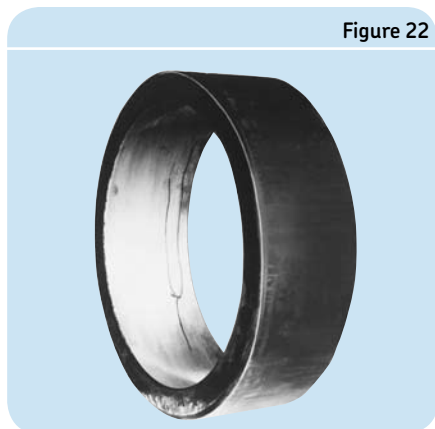
Cracks caused by faulty housing fit
