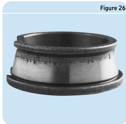
Fatigue caused by edge loading
