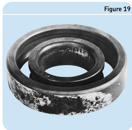
Wear due to fretting corrosion
