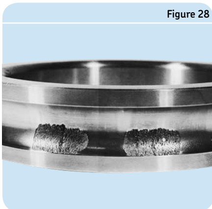
Fatigue caused by impact damage during handling or mounting
