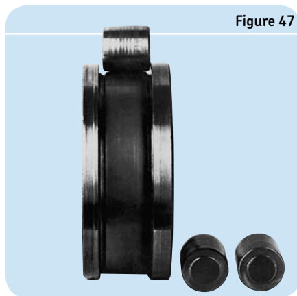
Grooves caused by wear due to inadequate lubrication
