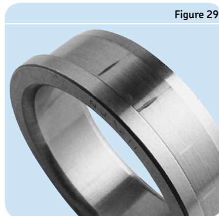
Smearing caused by excessive force in mounting
