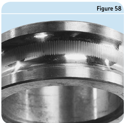
Fluting on raceway of ball bearing caused by prolonged passage of relatively small electric current
